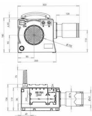
Unsurpassed in air quantity and air pressure at extremely small dimensions!
